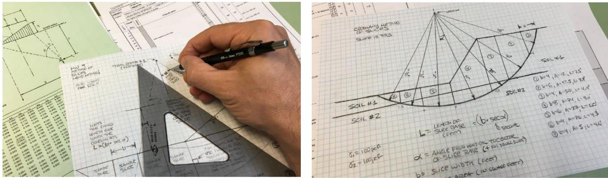
Figure 3: (a) Setting up a slope stability problem by hand (b) the finished slip surface evaluated by hand for one case using a simplified Ordinary Method of Slices evaluation.
