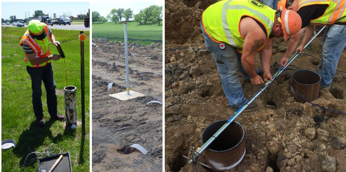
Figure 2: (a) A manual groundwater assesment using a weighted tape in a borehole piezometer; (b) a settlement plate to measure settlement in a field of prefabricated vertical drains; (c) and a series of rebar strainmeters attached to a centralizer bar before being placed in a concrete filled steel shell pile to measure strain distribution.
