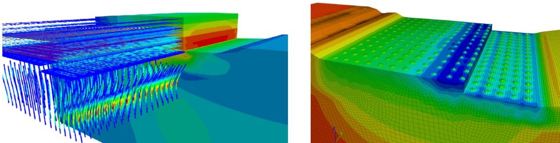
Figure 4: (a) Computer model of a column supported embankment (b) column supports
