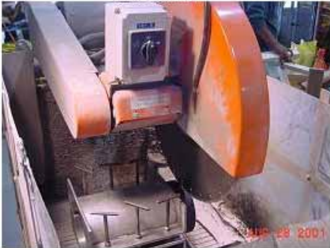
FIGURES 1 through 4 Initial steps in cutting gyrotory pill to obtain test specimens.
