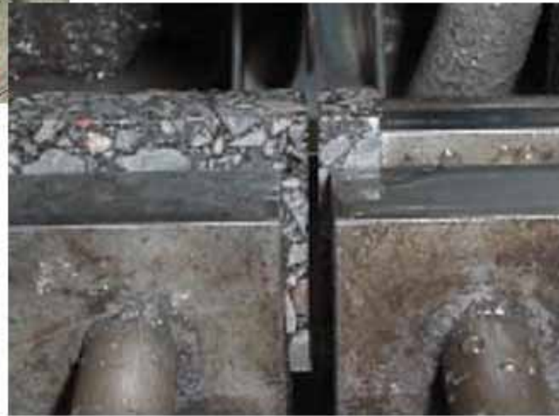
FIGURES 5 and 6 Cutting test specimen from rectangular section.
