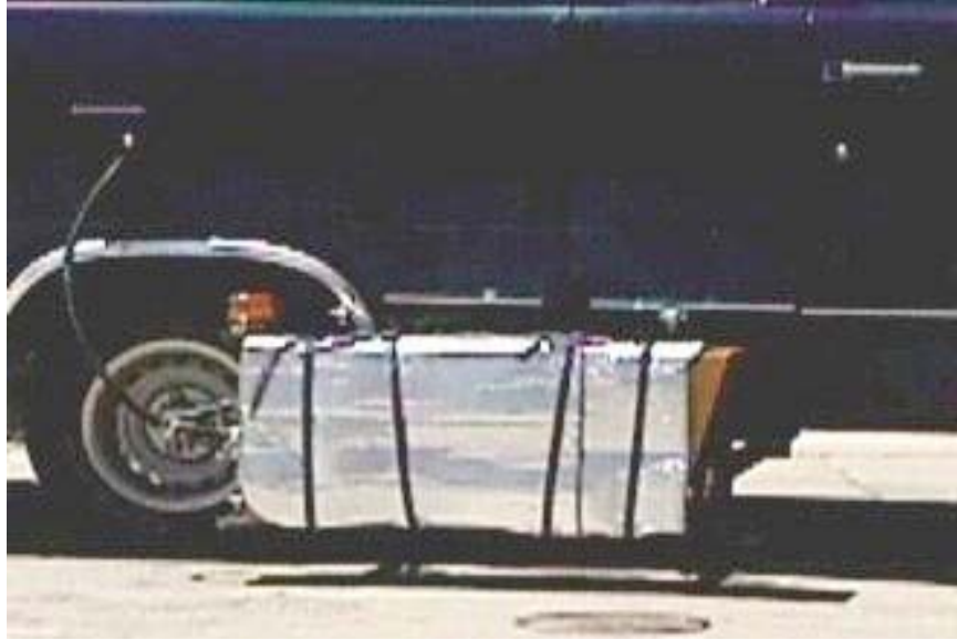
FIGURE 1 Laserlux mobile retroreflectometer mounted on a van.
