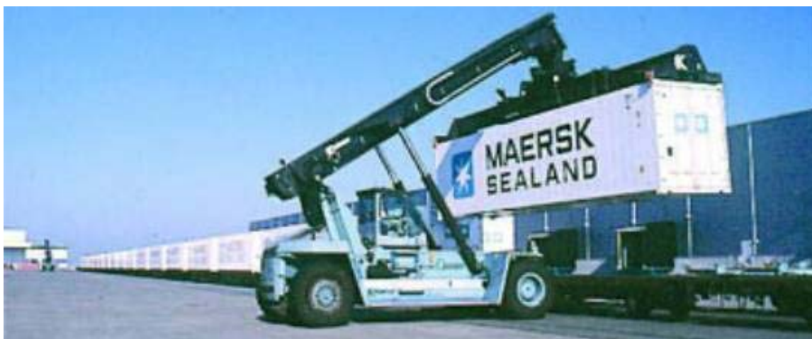
FIGURE 5 Top lifter used at APM Terminals, Port Elizabeth, New Jersey.
