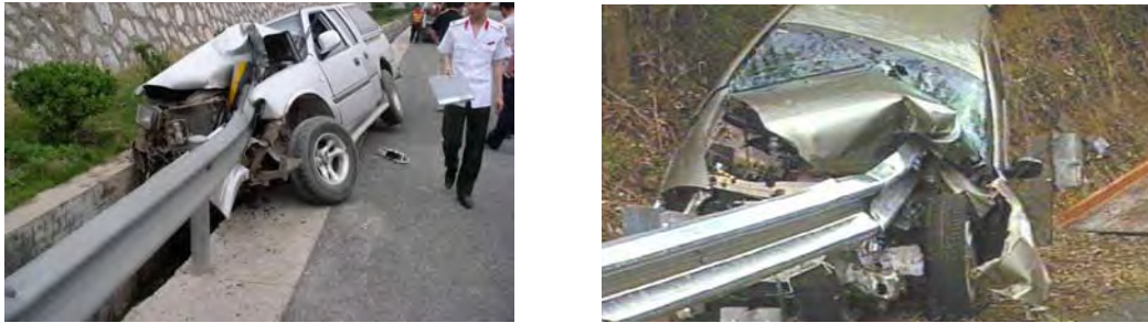
FIGURE 2 Unacceptable fishtail terminal performance.
