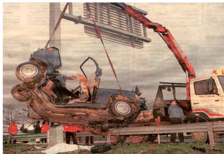
FIGURE 4 Vehicle after impact with turned-down end.
