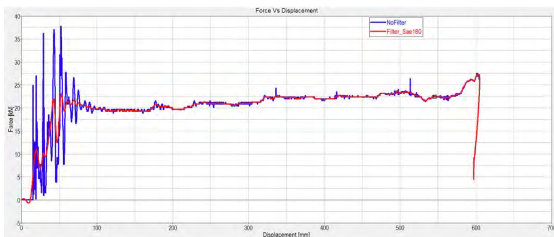
FIGURE 2 Force versus displacement curve for the steel honeycomb energy absorber. Blue curve: data from the calculation; red curve: SAE 180 filtered curve.
