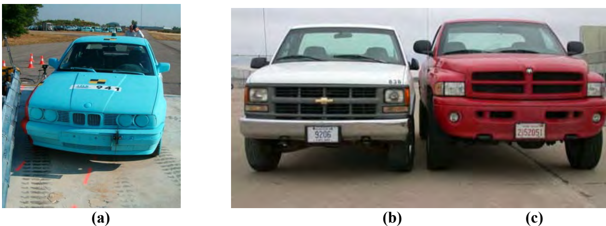
FIGURE 2 Larger test vehicles: (a) EN 1317, (b) NCHRP 350, and (c) MASH.
