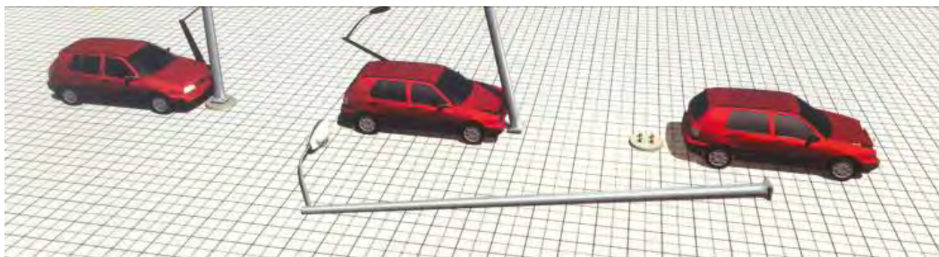
FIGURE 1 Breakaway pole collapse mechanism.
