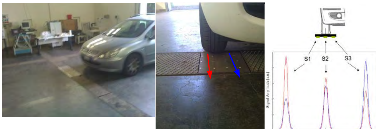
FIGURE 4 Experimental set-up for indoor WIM test at slow speed. Drawing on right shows dependence of sensors on position of transiting load: signals in red (blue) refer to load transiting on Sensor S1 (Sensor S3).
