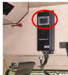
EMD F40 cab retrofit with Train Sentry III visual alert above forward view
