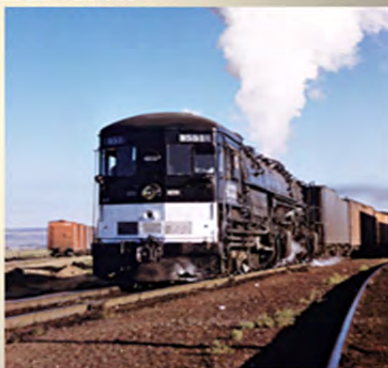
SP - Baldwin - Cab-forward design 1909 - 1940s
