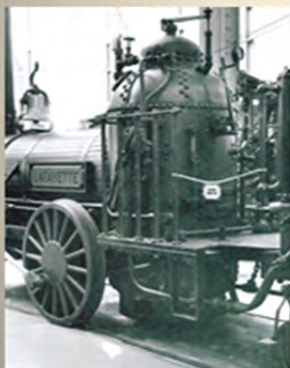
B&O – W. Norris & Co. - Lafayette horizontal boiler with no cab 1837 -
