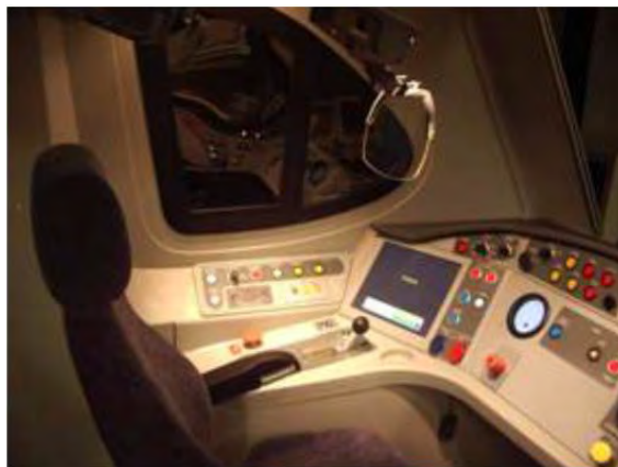
FIGURE 1 HUD fitted to a full-task train simulator.
