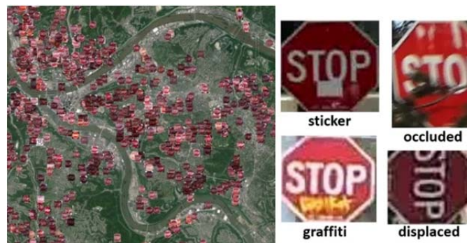
FIGURE 3 A map of stop signs detected in Pittsburgh and four individual signs with problems: defacement, occlusion by vegetation, and displacement.
