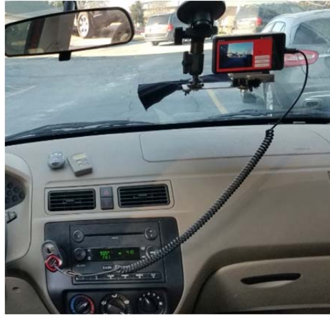
FIGURE 1 Smartphone mounted on windshield of vehicle collects images, GPS, and other sensor data.
