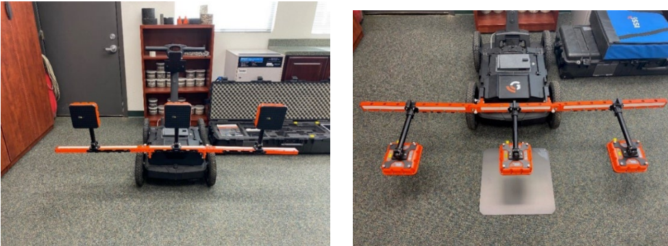
FIGURE 47 Performing the air and metal plate calibration process.
