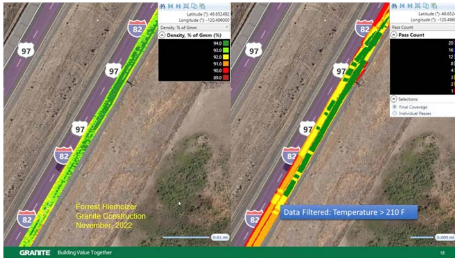
FIGURE 10 Example showing project meeting Caltrans specification.
