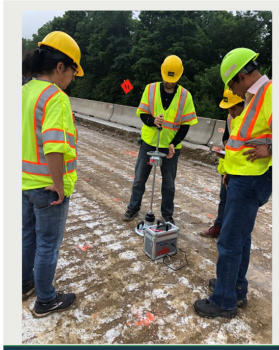
FIGURE 3 Quality assurance by agency staff using lightweight deflectometer.
