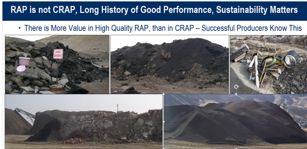
FIGURE 8 Importance of RAP quality and consistency for high RAP mixture production.
