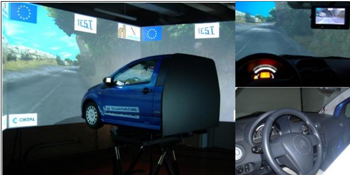
Figure 1 The VERA driving simulator
