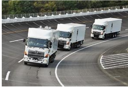
Figure 5 Automated platoon system for heavy trucks in Japan
