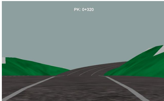
Figure 2: Screen from AVI video – “optical break” shortcoming Font: CLIP software, modified by author
