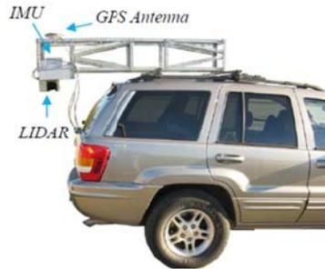
Figure 2: Instrumented Vehicle for Data Collection (Vemulapalli and Brennan, 2009)
