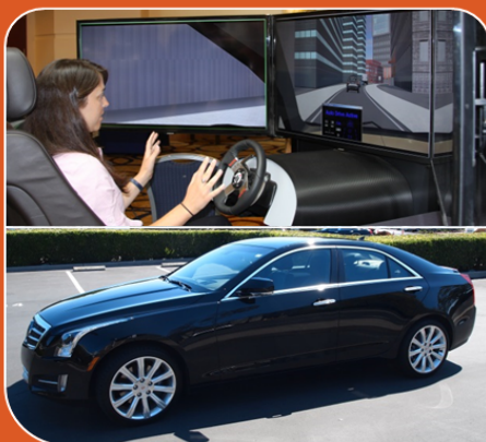
Magna demonstrated a monocular camera-based Traffic Jam Assistance system, capable of automatically operating in stop and go traffic at speeds up to 44 mpg (bottom). Magna also demonstrated this same system with the use of a simulator inside the symposium (top).
