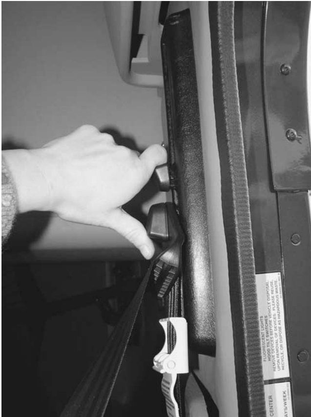
Figure 9. Shoulder strap D-loop height adjuster.
