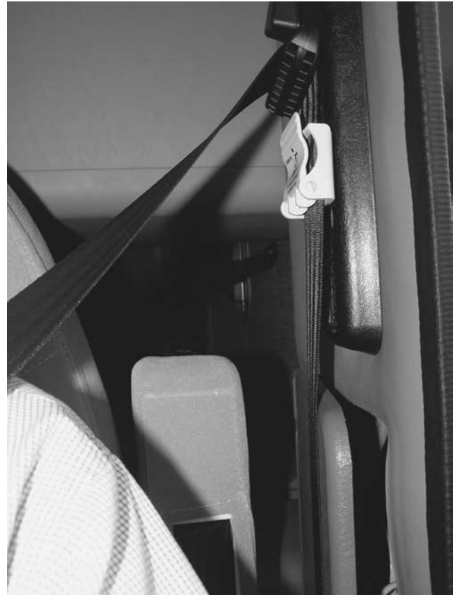
Figure 11. Shoulder strap tension adjustment mechanism (latched).
