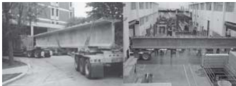
Test girders arrive at Newmark Laboratory, University of Illinois, for NCHRP Project 12-56, Application of the LRFD Bridge Design Specifications to High-Strength Structural Concrete: Shear Provisions (from NCHRP Report 579).
