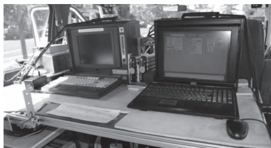
Computer monitors on board a mobile data collection van participating in the September 2008 SHRP 2 rodeo, which evaluated the precision and accuracy of mobile roadway measurement and pavement data collection systems for Project S-04: Acquisition of Roadway Information.
