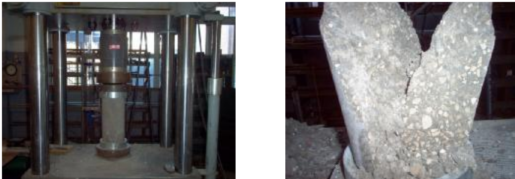
Fig. 2.8 MTS machine and destructive concrete sample
