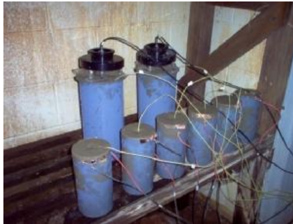
Fig. 2.3 a) schematic of tube sensor accommodating the cylinder specimen; b) photo of monitoring channels
