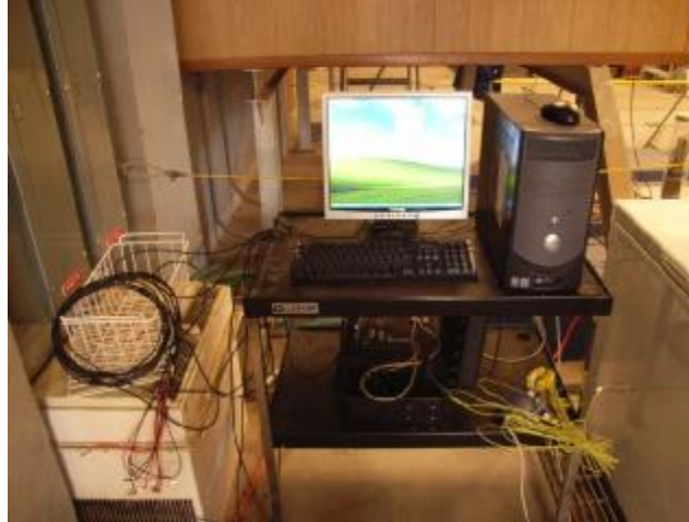
Fig. 2.4 monitoring station for curing concrete
