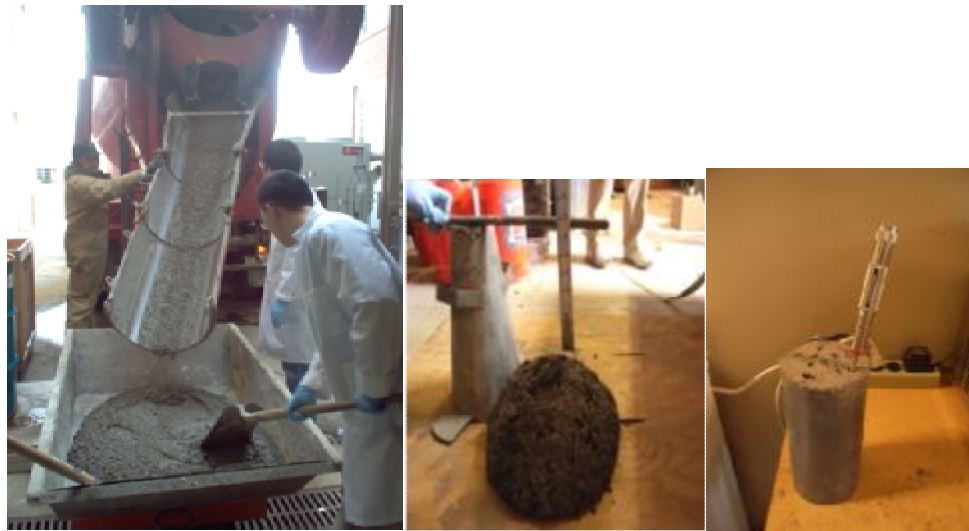
Fig. 2.5. Photo of concrete delivery, slump test and penetration test
