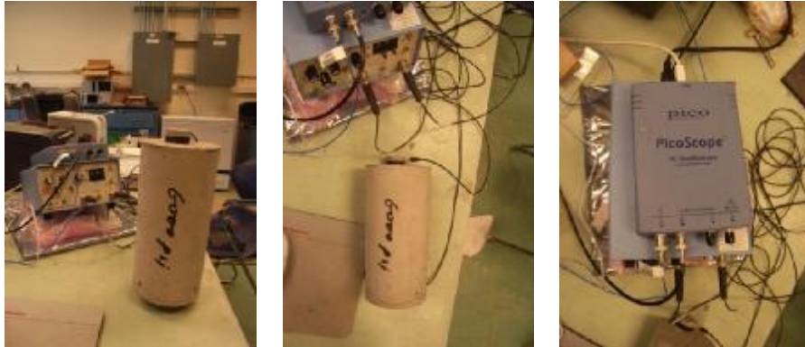
Fig. 2.7 Ultrasonic testing device and example photos of testing concrete specimen
