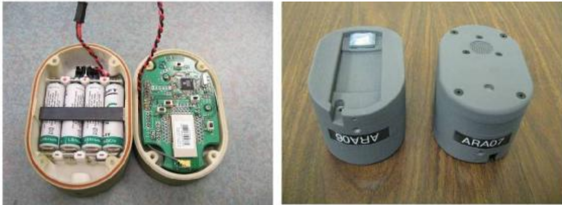
FIGURE 4: Photos of the SSAM units. LEFT—Inside the enclosure is housed four batteries and the circuit board. RIGHT—Top and bottom views of the SSAM sensor .
