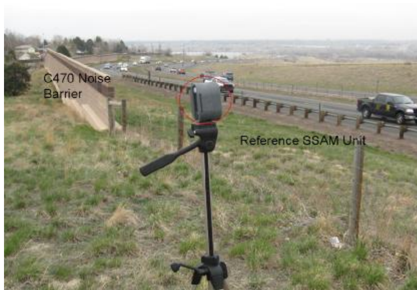
FIGURE 11: Equivalent before site reference microphone position. The reference SSAM is 1.5 m above the ground and about 4 m above the nominal plane of the sound source.
