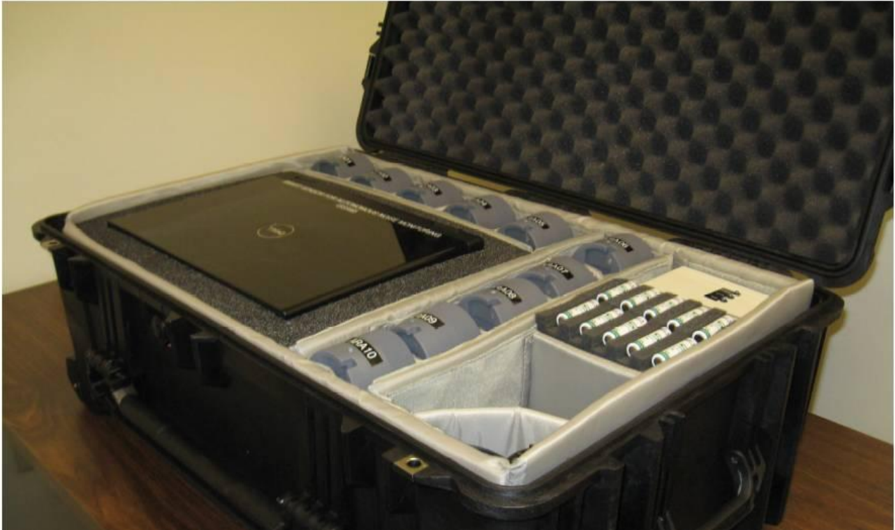
FIGURE 5: Photograph of the completed sensors and base station stored in their travel case. The case contents include: laptop, ten SSAMs, one USB receiver module with short range receiver antenna, cord and power supplies, and replacement batteries. Not shown is the larger optional receiver antenna used for longer range wireless reception.
