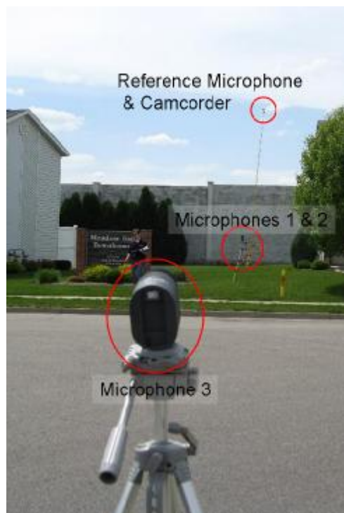
FIGURE 13: Photograph taken from behind microphone 3 facing the noise barrier.
