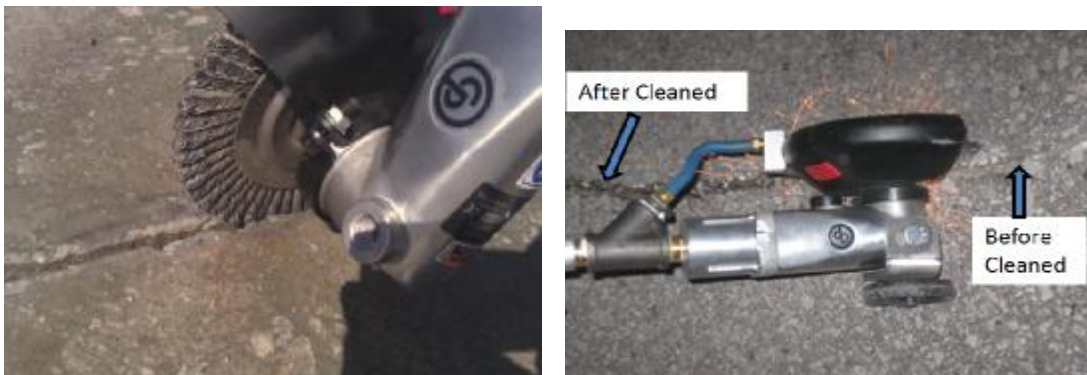
FIGURE 12: Twisted wire narrow faced brush test.
