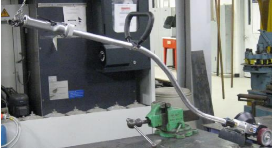
FIGURE 17: Finalized shaft design.
