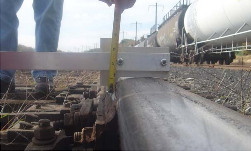
Figure 17: Chipped point as measured by Gauge 2
