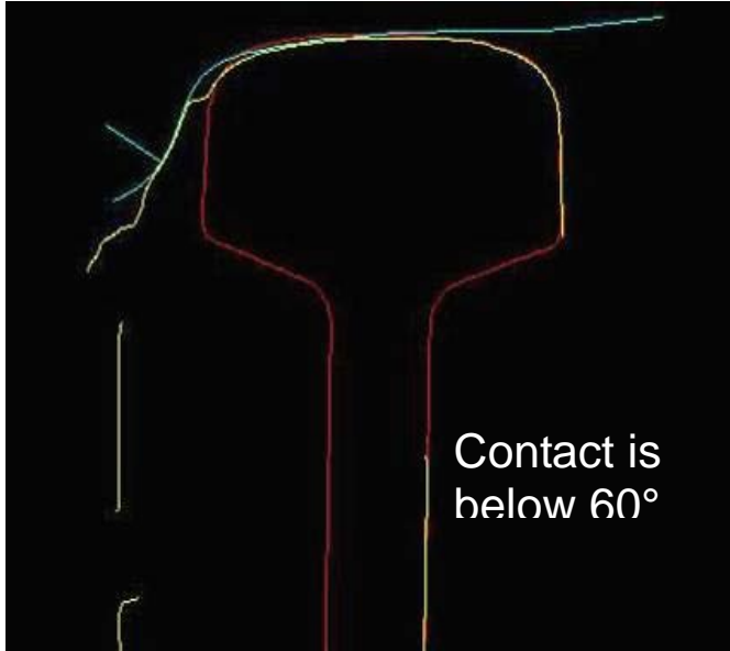
Figure 3: Flange contact below 60° mark
