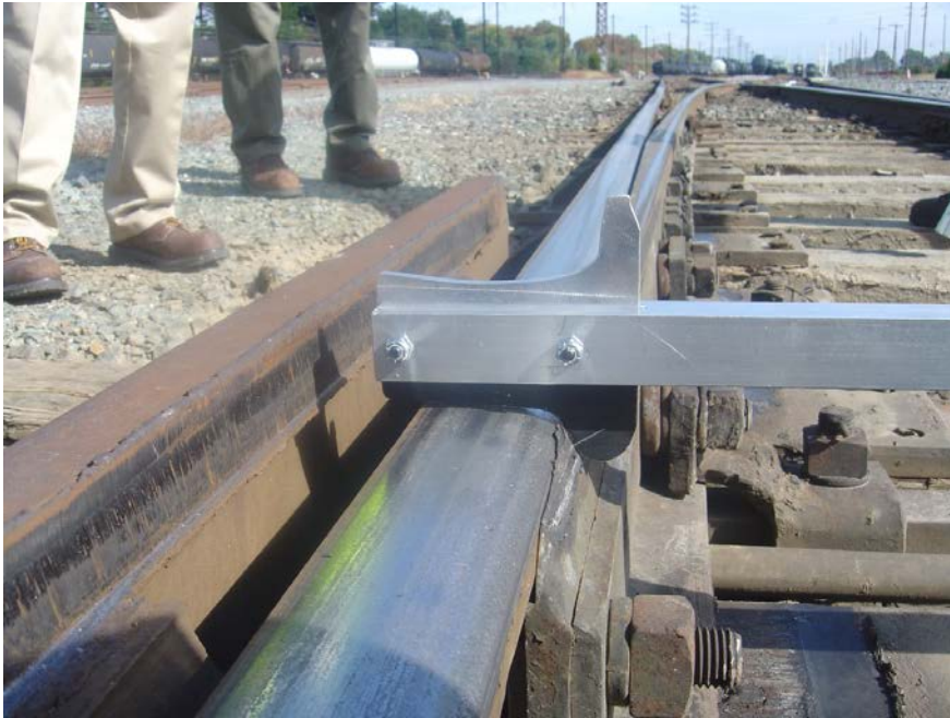
Figure 19: Modified Wheel Profile Gauges during evaluation
