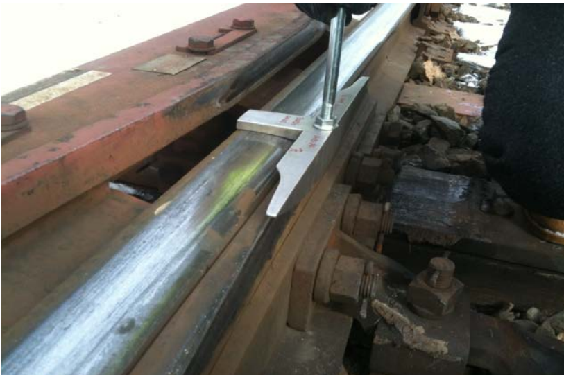
Figure 23: “Half Moon” gauge with Moderately Worn Wheel Segment
