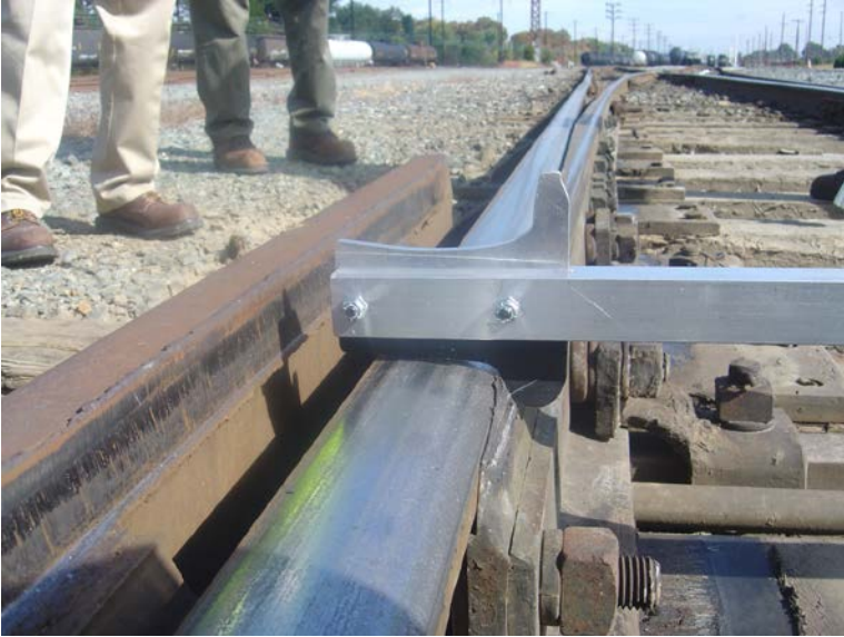
Figure 16: AAR 1B Wheel Profile Gauge as manufactured in the US by Norfolk Southern (bottom, on switch point) with severely worn US profile gauge in top position.
