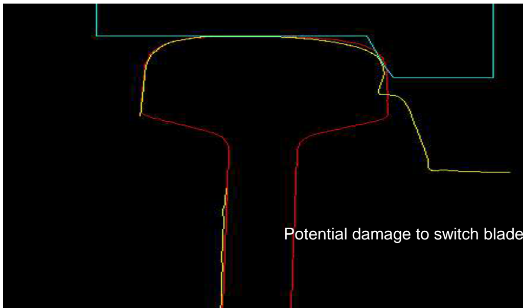
Figure 8: Switch rail with damage that fails Gauge 2 inspection
