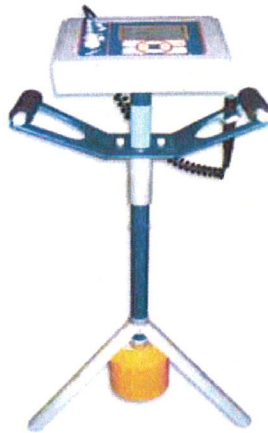
Briaud compaction device (BCD)
