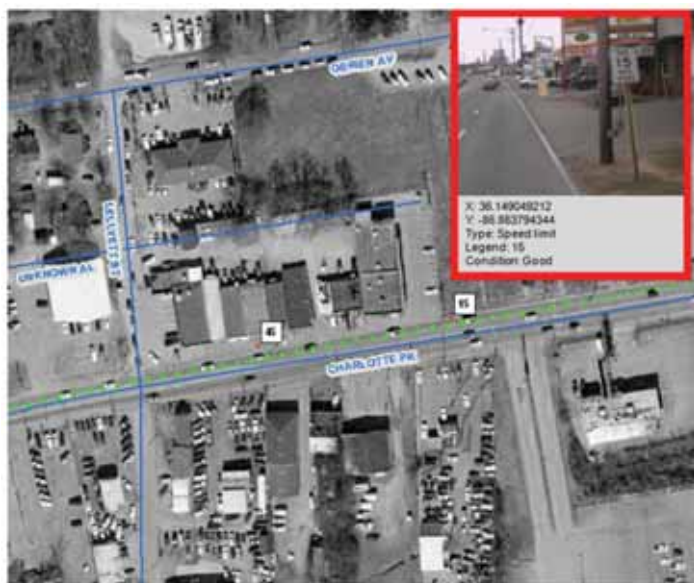
Traffic signs can be automatically extracted from video images and labeled onto a Google map so transportation agencies know where their sign assets are.
