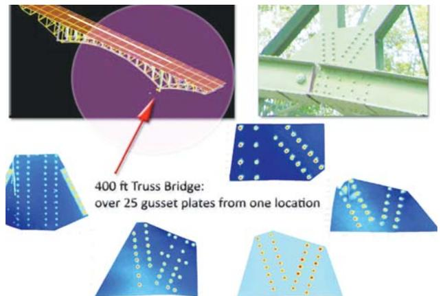
The laser metrology instrumentation system can measure *many* bridge details from one laser position.
