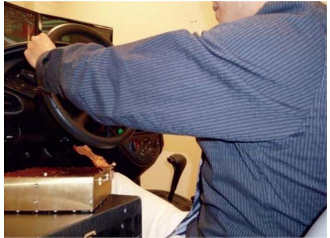
The sensor (left) monitoring a driver in a simulated vehicle cab.
