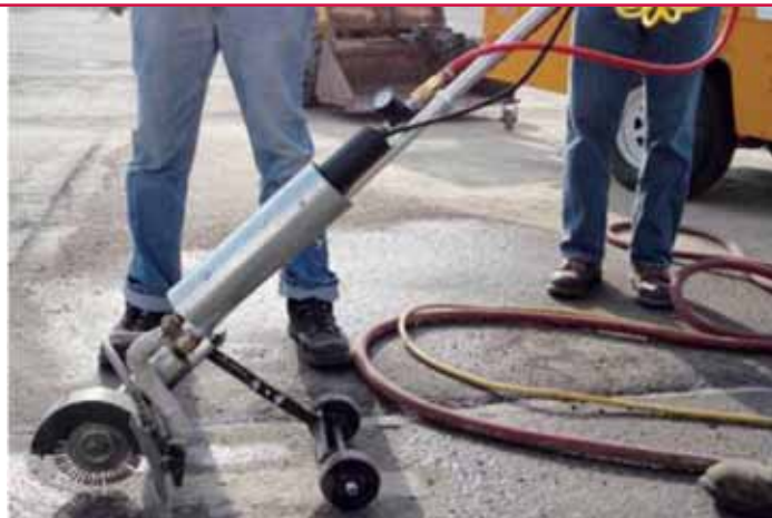
Crack Cleaning Device (CCD) with Heat Lance Attachment in Field Test with Nebraska Department of Roads Crew
