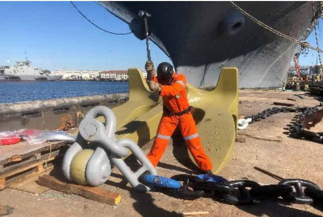
Assembling emergency anchor in advance of tow.
