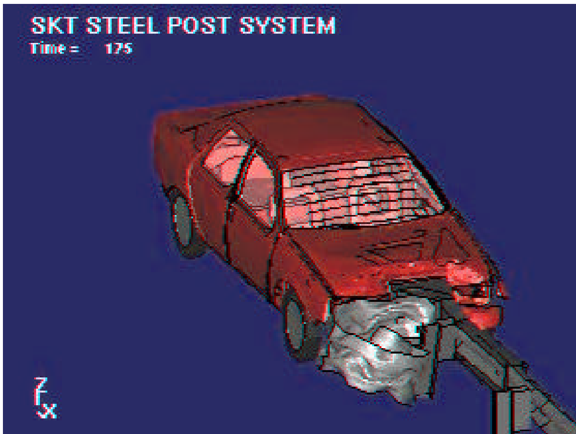
FIGURE 1 Computer simulation of a guardrail terminal impact.
