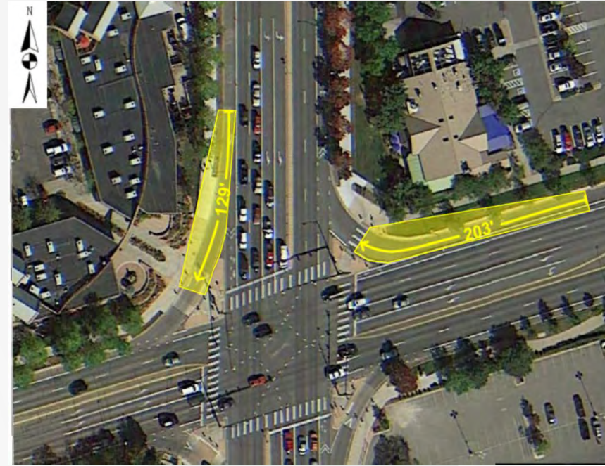
Illustration of Sight Distance for CTL with and without raised crosswalk
