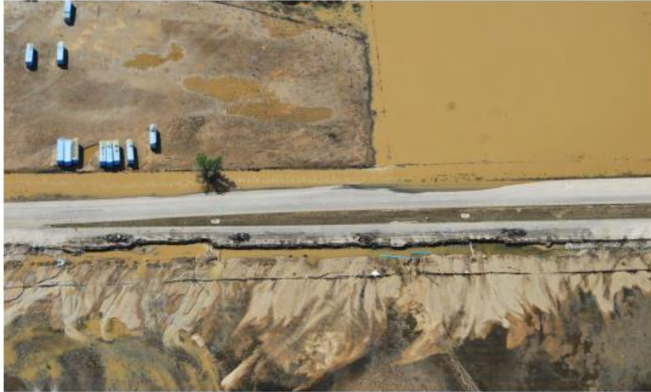
Figure 26 - MP 62.8, Aerial photo, Damaged roadway and shoulder with evidence of overtopping
