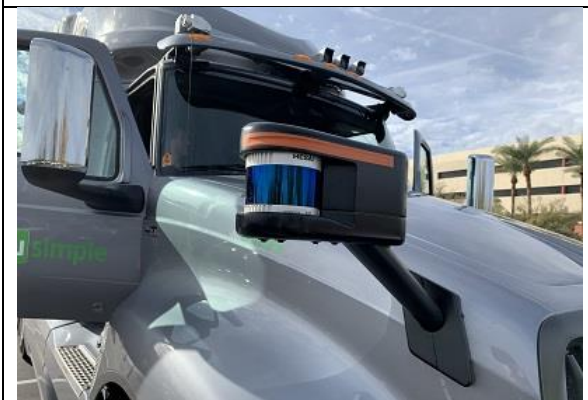
LiDAR device on a TuSimple automated truck, Dec 2019, Chandler (AZ)
