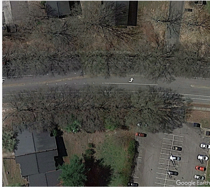
Bicycle path departing bike lane and crossing vehicle lane for left turn downstream.
