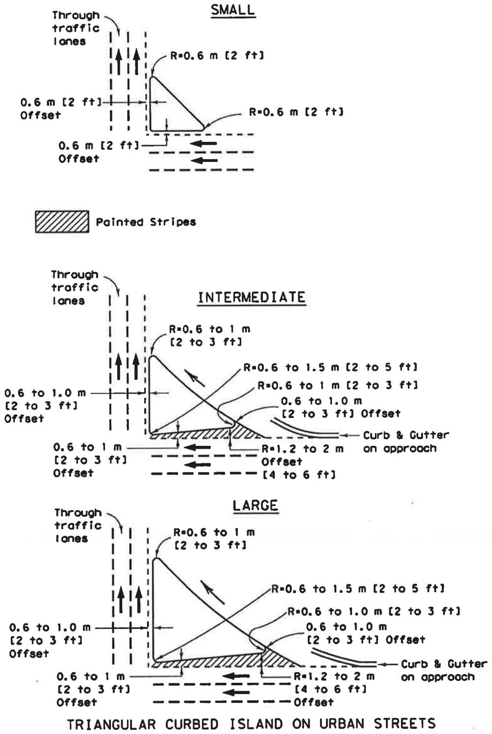
Figure 4. Details of corner island designs for turning roadways at urban locations (1, 2).
