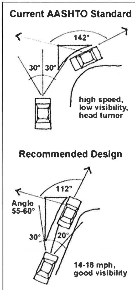
Figure 6. Current and recommended design of entry angle for channelized right-turn lane (10).
