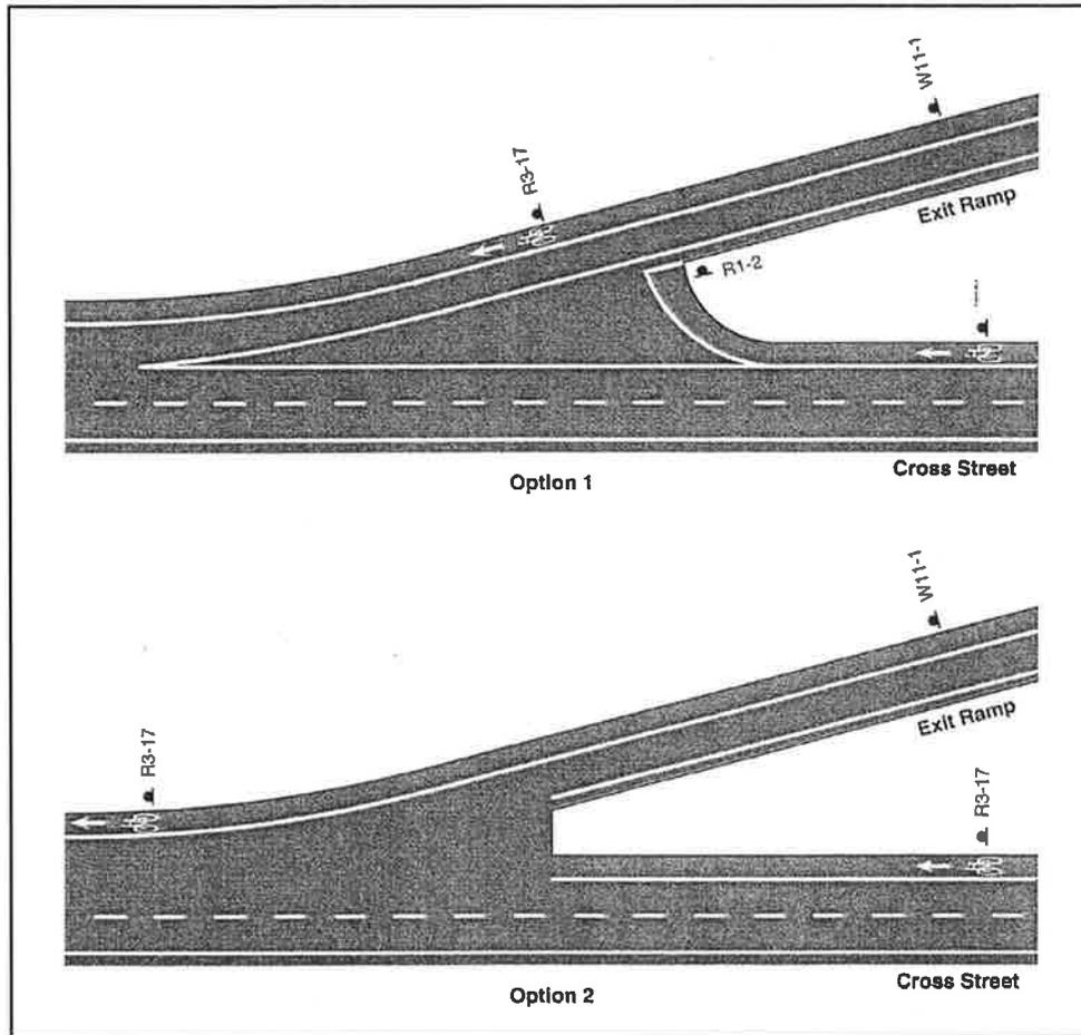
Figure 17. Bicycle lanes crossing interchange exit ramps (14).
