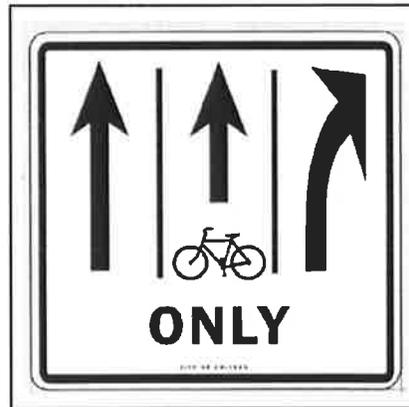
*Figure 13. Standard signing for bicycle lane at intersection (18).*
