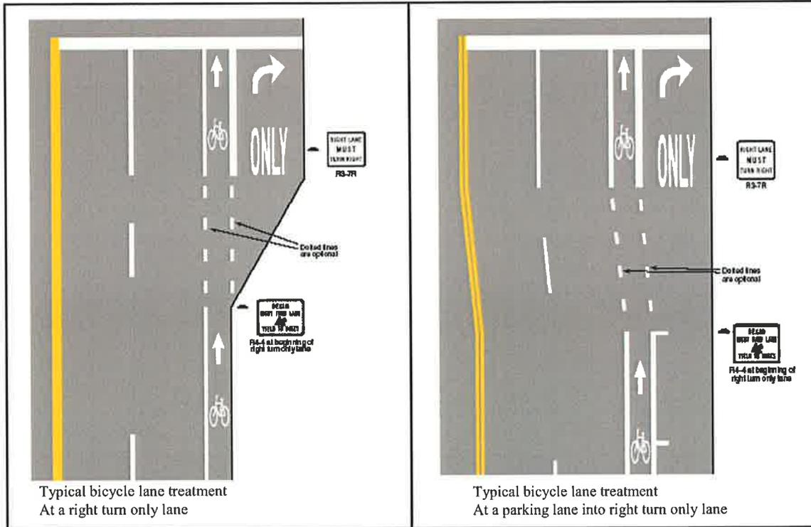
Figure 10. Typical intersection pavement markings (11).
