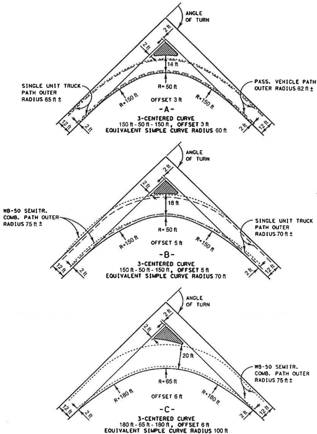
Figure 5. Minimum Turning Roadway Designs With Corner Islands at Urban Locations (1, 2)
