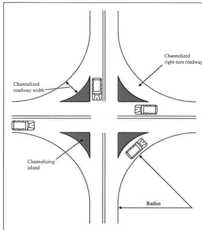
Figure 1. Typical intersection with channelized right turns.
