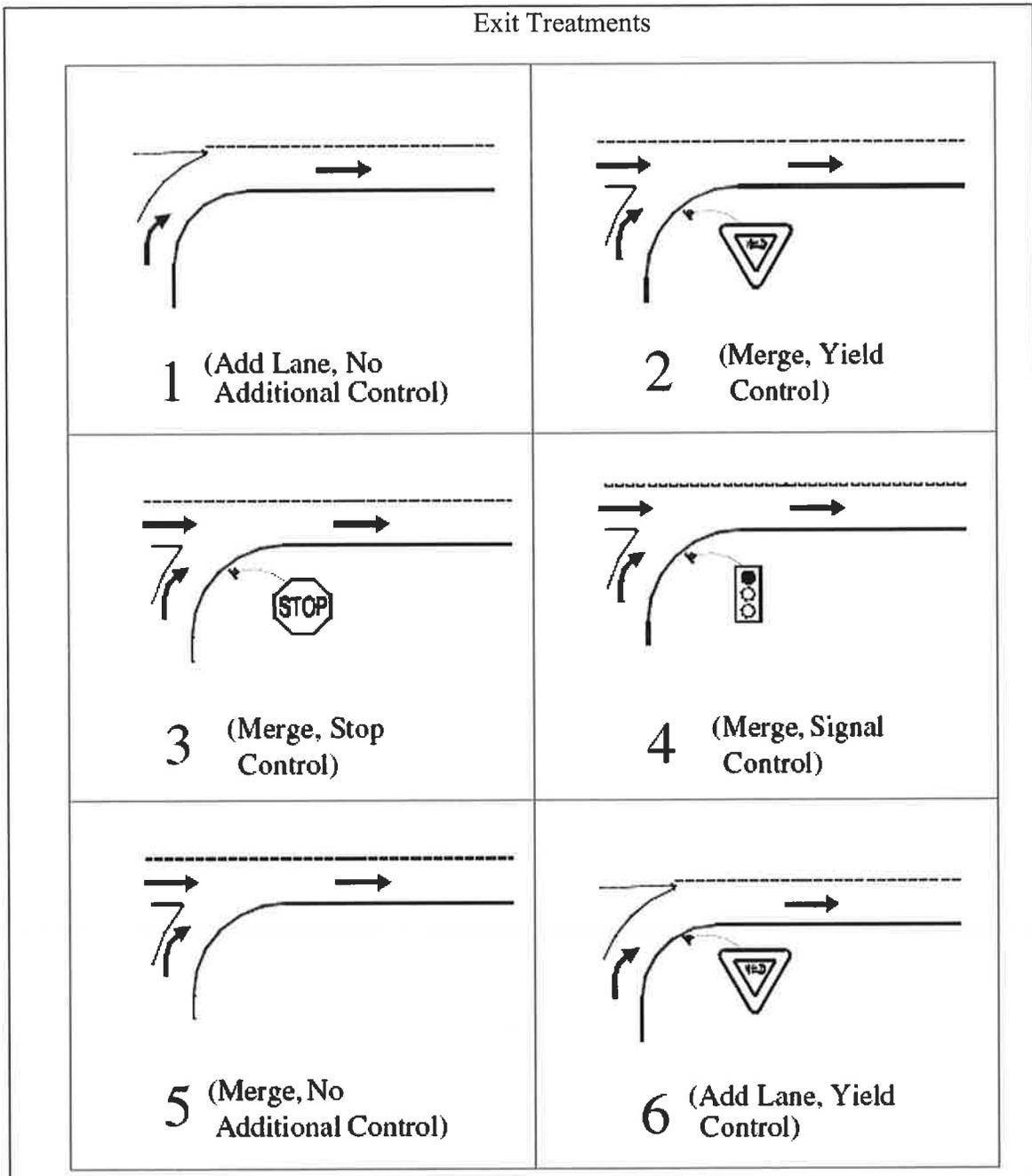
Figure 3. Geometric and traffic control treatments for the downstream or exit end of channelized right-turn roadways (4).
