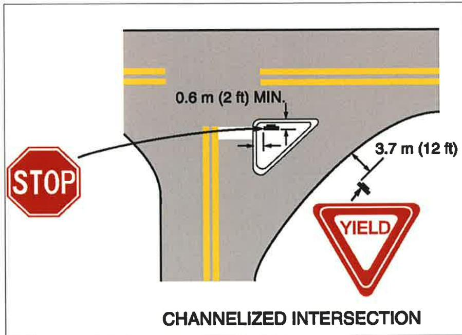
Figure 8. Typical locations for signs at channelized right turns (11).
