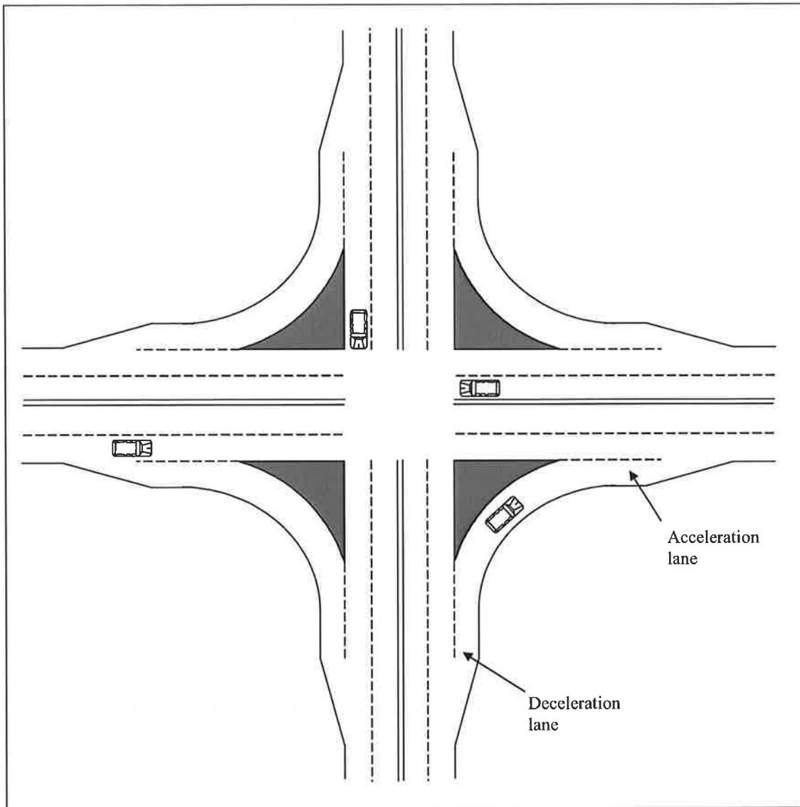
*Figure 7. Channelized right turns with deceleration and acceleration lanes.*
