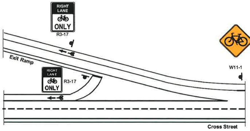
Figure 14. Bicycle crossing of interchange ramp (17).
