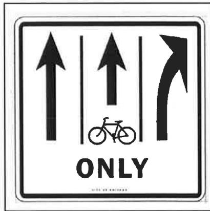
*Figure 9. Standard signing for bicycle lane at intersection (7).*
