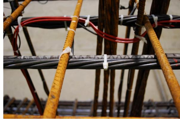
(e) Instrumented embedded top bar
