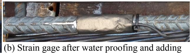
(b) Strain gage after water proofing and adding “mechanical” protection
