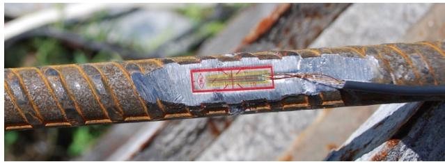
(a) Strain gage on a non-prestressed longitudinal reinforcing bar
