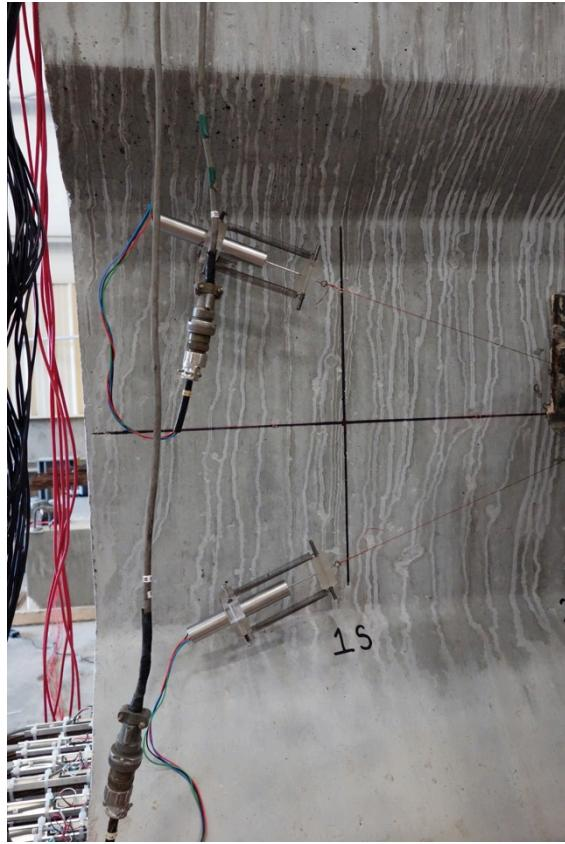
**Figure G.7.** Diagonal displacement transducers
