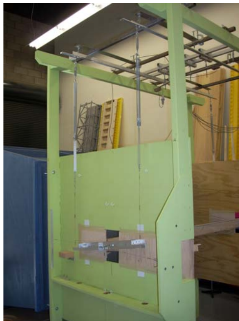
Figure 3-10 – End Support of Beams during Wind Tunnel Testing
