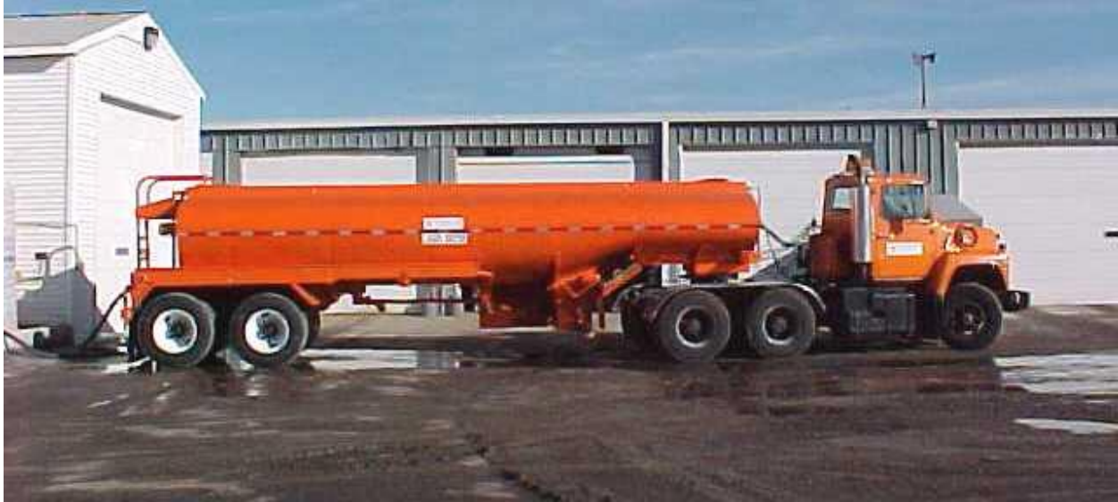
Figure 3. 5000 Gallon Tanker for Brine Application on Interstate Highways.
