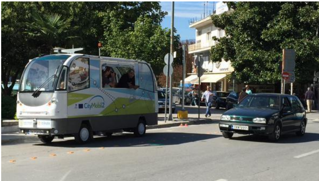
Figure 3. CitiMobil2 Demonstration Projects – Vehicles Operated in Protected Lanes at 20 kph and in Mixed Traffic at 10 kph
