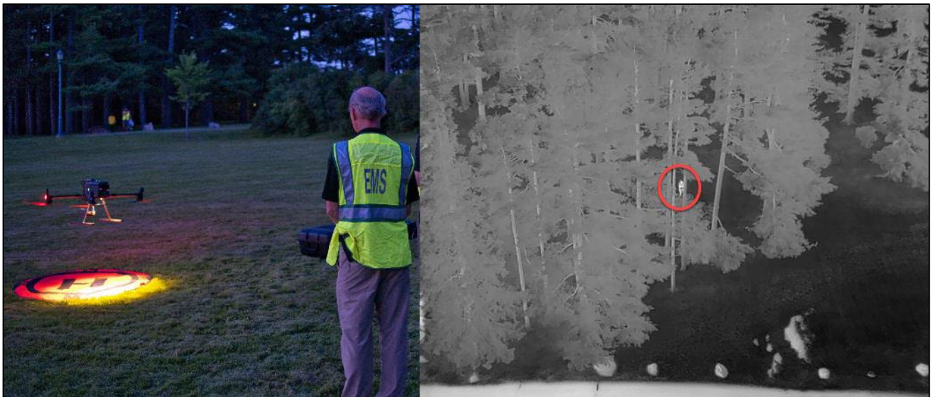
Figure 10: A pilot conducts a search & rescue simulation to locate a person using a high-resolution thermal sensor (right)
