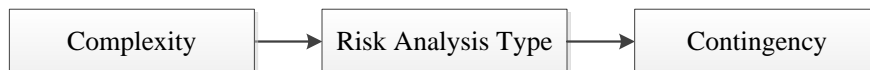
Figure 7 The Three Tier Approach Process to Estimate Project Contingency Adopted "A risk-based approach to contingency estimation in highway project development" (Molenaar and Wilson 2009)
