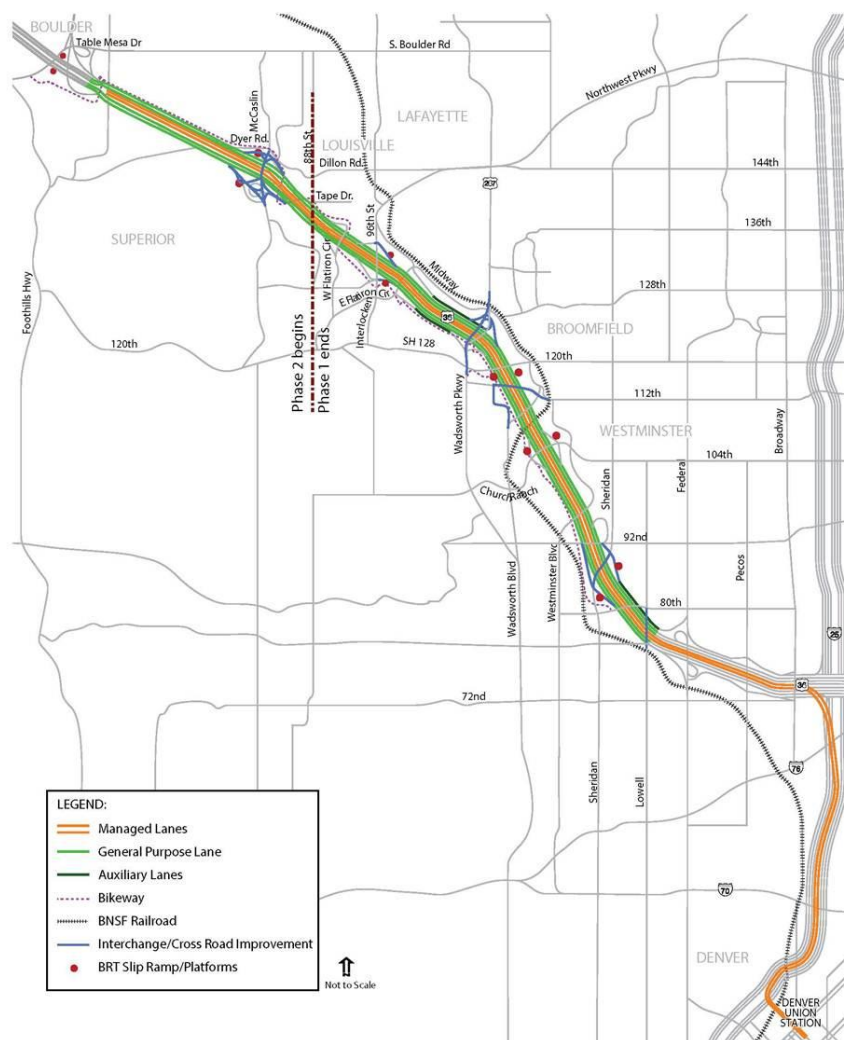
Figure 4-4 US 36 Managed Lane/BRT Corridor
