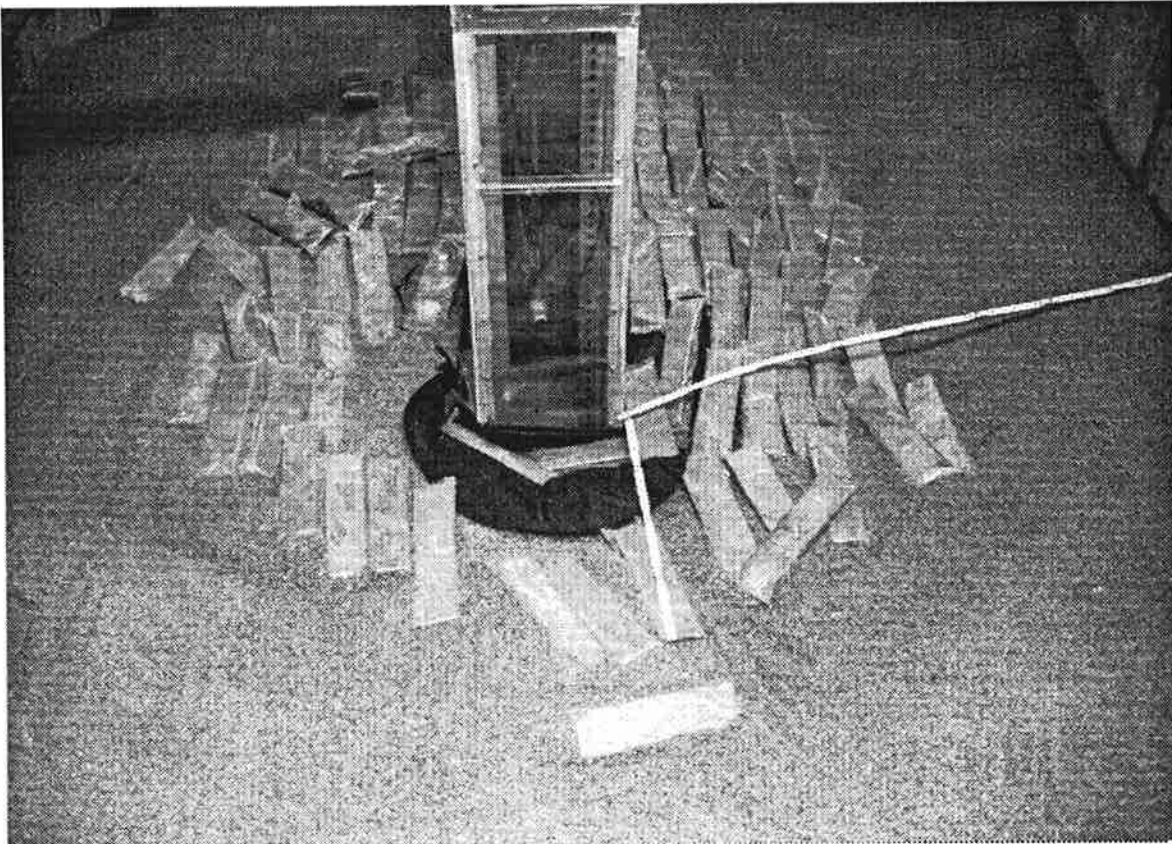
Figure 8.8c. Illustration of the dispersive sliding of grout filled bags under conditions for which the equivalent riprap did not fail.
