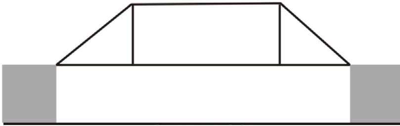
Figure 3-6. Elevation drawing of queen post truss.
