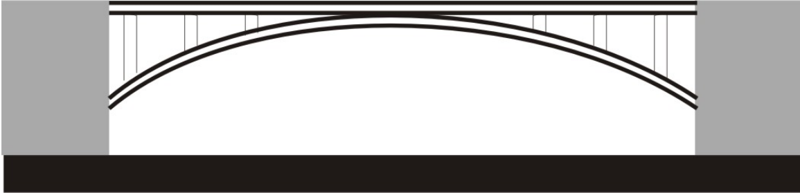
Figure 3-56. Elevation drawing of open spandrel concrete arch.
