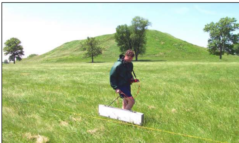
Figure 8. Electromagnetic conductivity survey in progress. Image from (Clay 2006:80).
