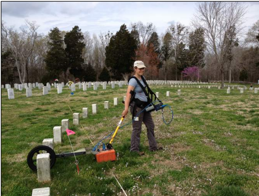
Figure 5. Ground-penetrating radar survey in progress. Image source: New South Associates.
