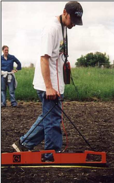
Figure 9. Slingram instrument being used to collect susceptibility data. Image from (Dalan 2006:168).
