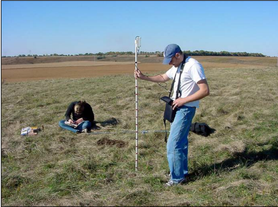
Figure 11. Down-hole magnetic susceptibility meter (Dalan 2006:169).
