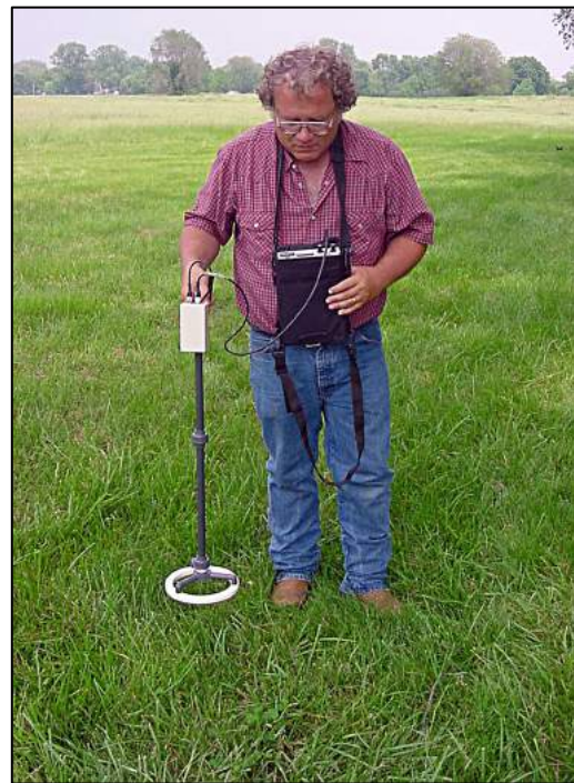
Figure 10. Single-coil susceptibility meter. Image from (Dalan 2006:168).
