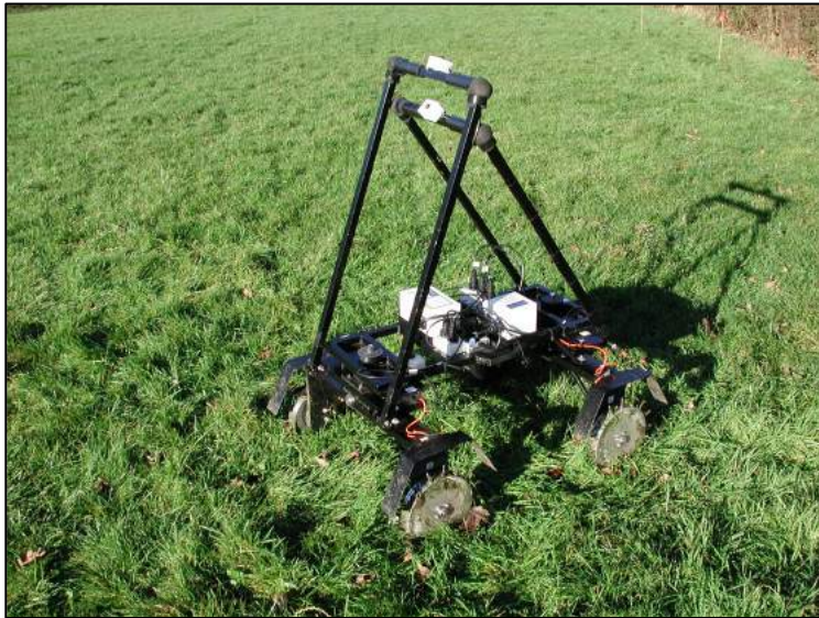
Figure 7. Square array resistivity configuration. Image from (Somers 2006:116).
