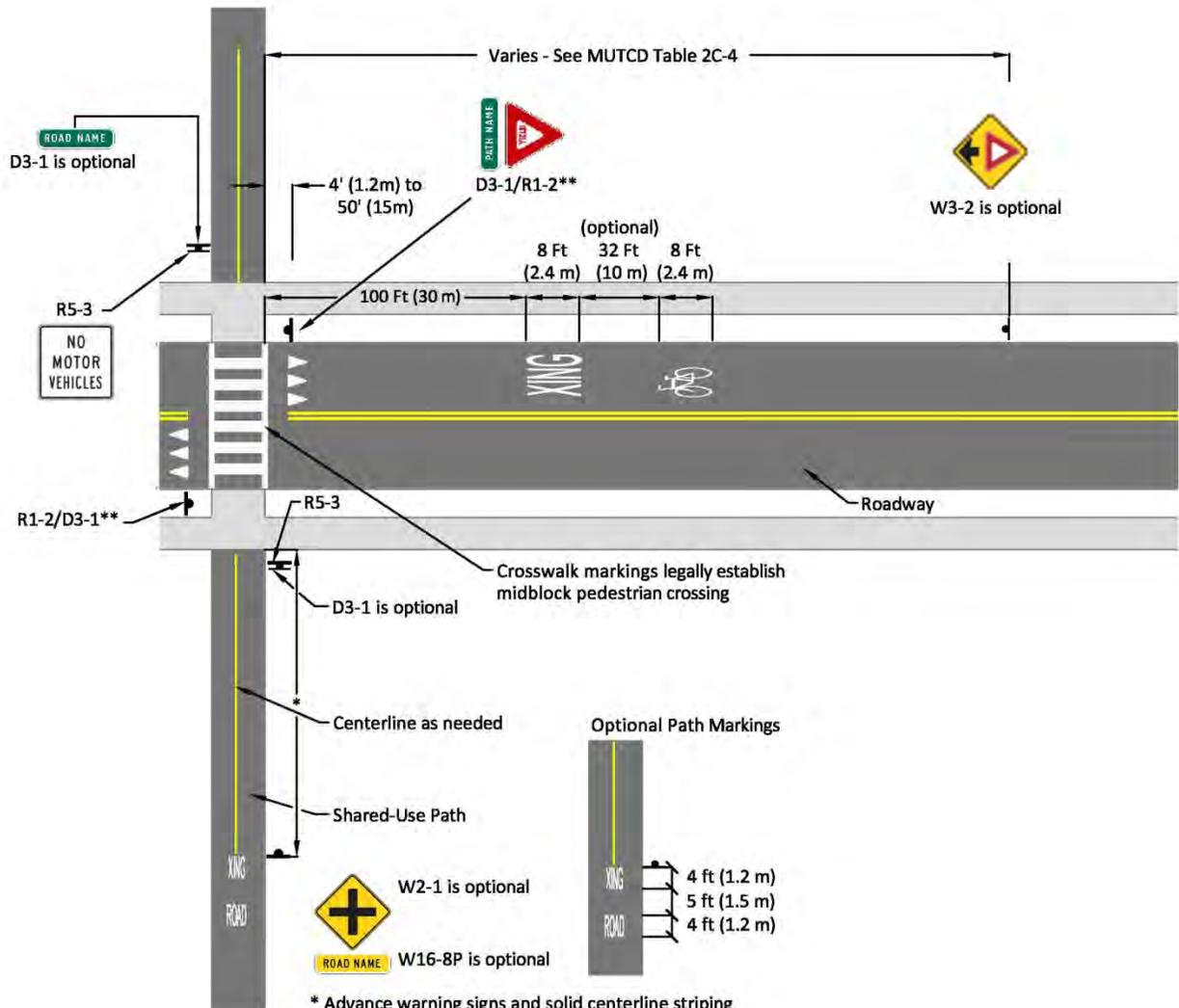
\* Advance warning signs and solid centerline striping should be placed at the required stopping sight distance from the roadway edge but not less than 50 feet (15m).
