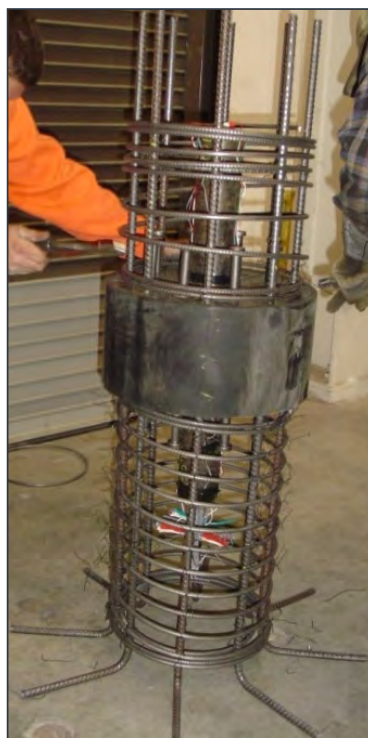
Figure 2.46 Details of rubber pad incorporated into a segmental column model at UNR
