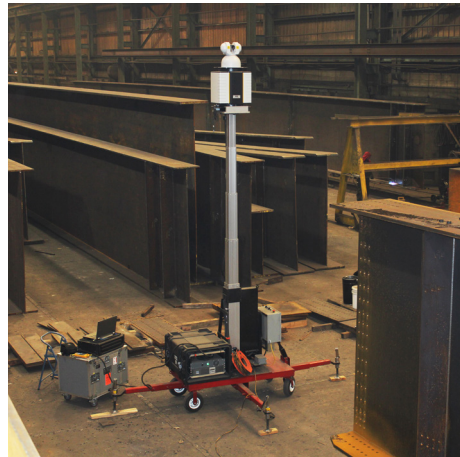
The Bridge Virtual Assembly System's laser detection allows bridge girders to be fitted via a computer model rather than manually in fabrication shops.
