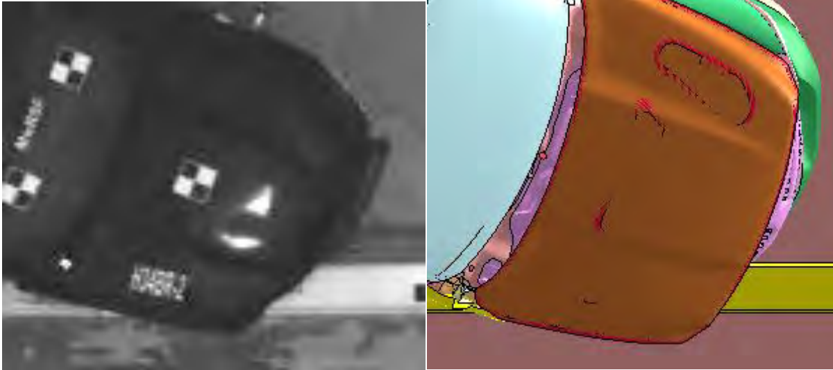
Figure D-18. Maximum Lateral Extent during Test No. H34BR-2 (Bielenberg 2019) and Simulation
