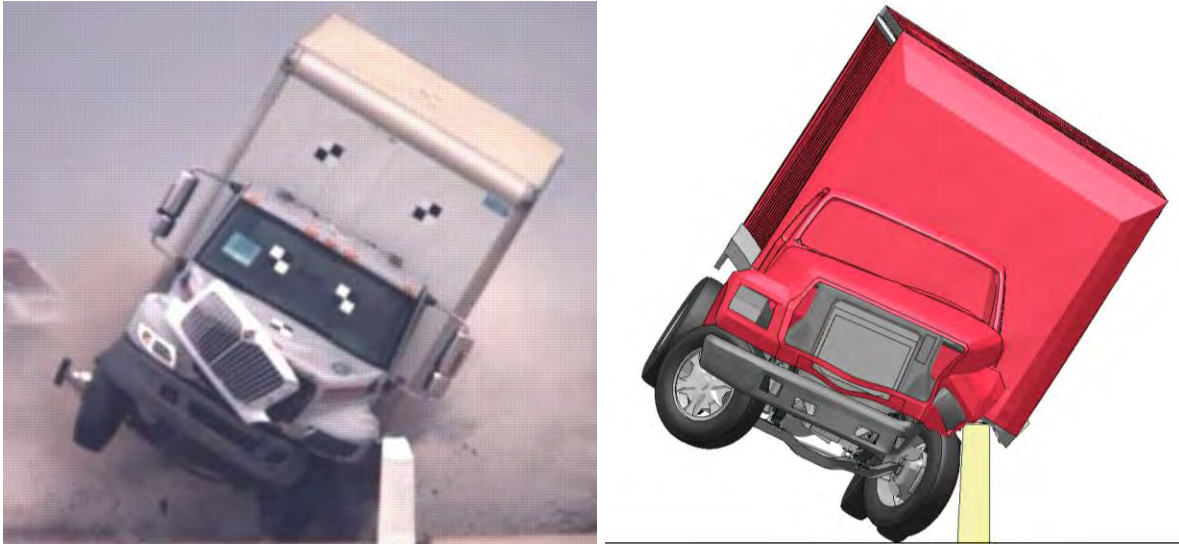
Figure E-11. Maximum Lateral Extent during Test No. 4CBR-1 (Rosenbaugh et al. 2021) and Simulation
