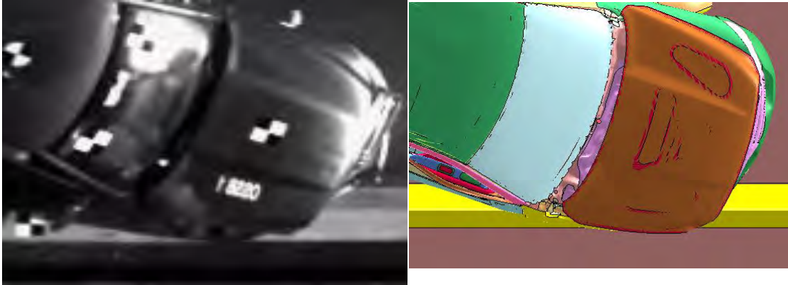
Figure D-30. Maximum Lateral Extent during Test No. OSSB-1 (Bielenberg, Faller, and Ronspies 2018) and Simulation
