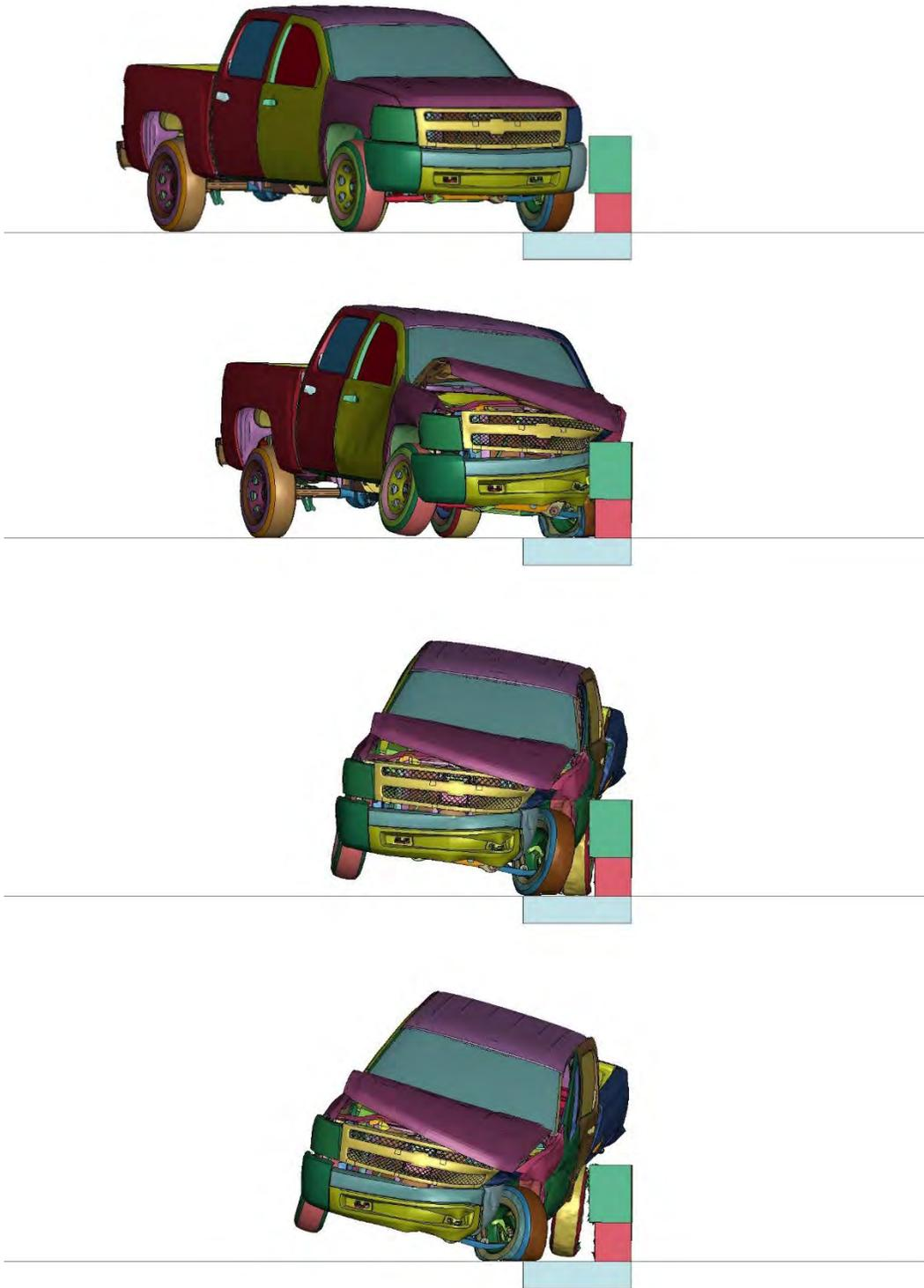
**Figure C.27. Key sequential gut view of MASH Test 3-11 on the Kansas Corral system at midspan.**
