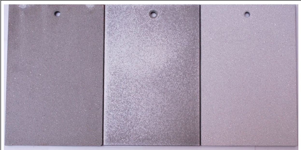
AI TSC: Humidity exposed (L), Humidity exposed with power sand (C), No exposure (R)
