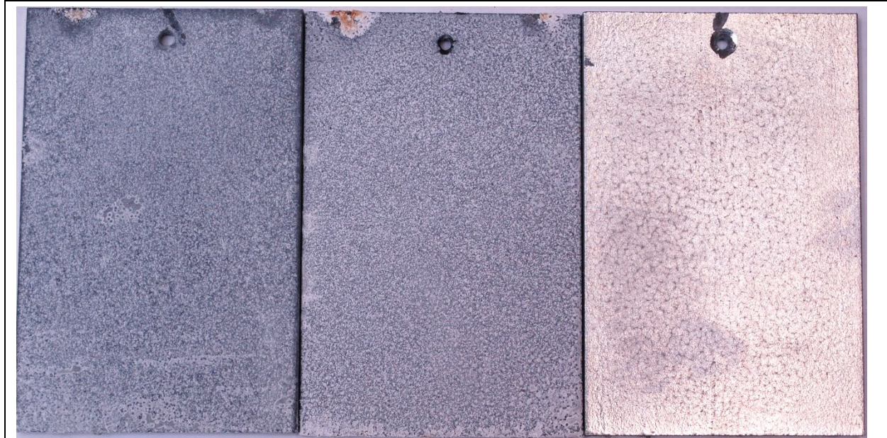
HDG: Prohesion exposed (L), Prohesion exposed with SP 1 (C), No exposure
