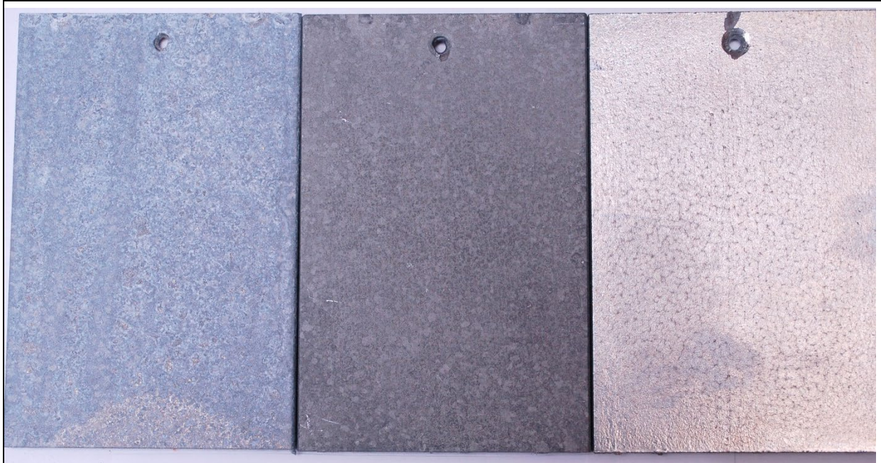
HDG: Humidity exposed (L), Humidity exposed with SP16 (C), No exposure (R)
