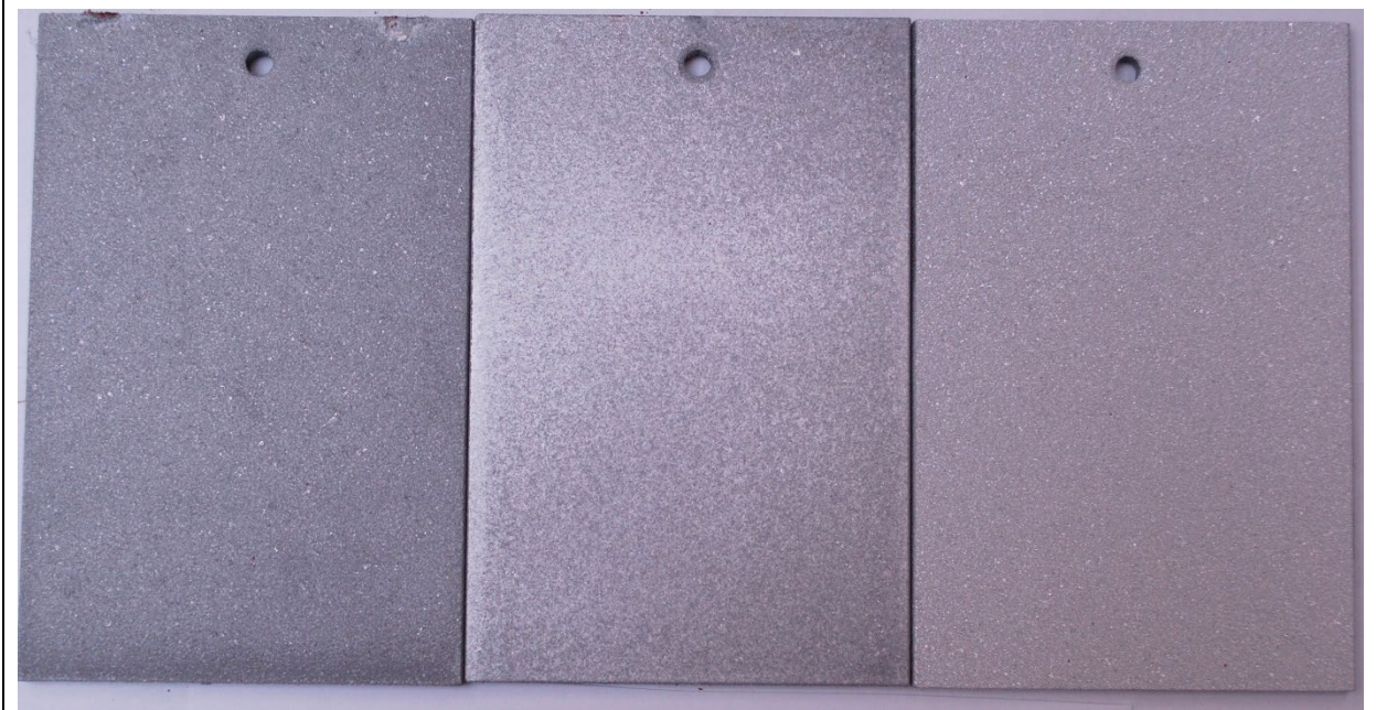
AI TSC: Prohesion exposed (L), Prohesion exposed with power sand (C), No exposure (R)
