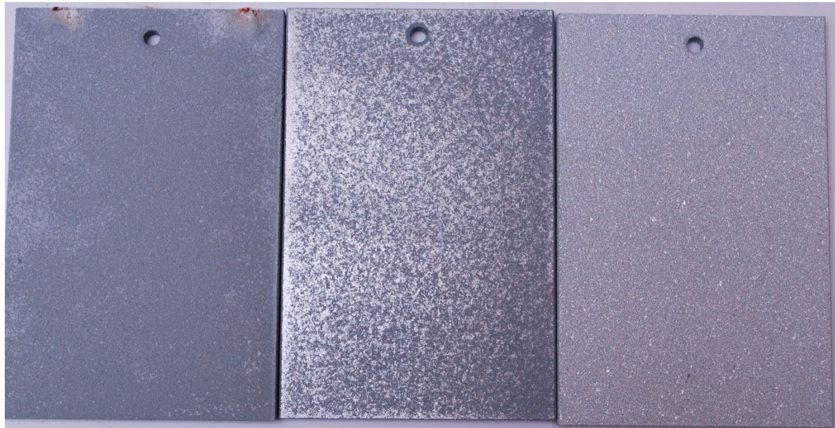
Zn TSC: Prohesion exposed (L), Prohesion exposed with power sand (C), No exposure (R)
