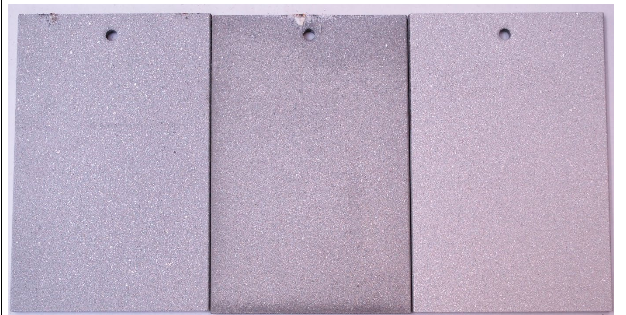
AI TSC: Cohesion exposed (L), Cohesion exposed with SP1 (C), No exposure
