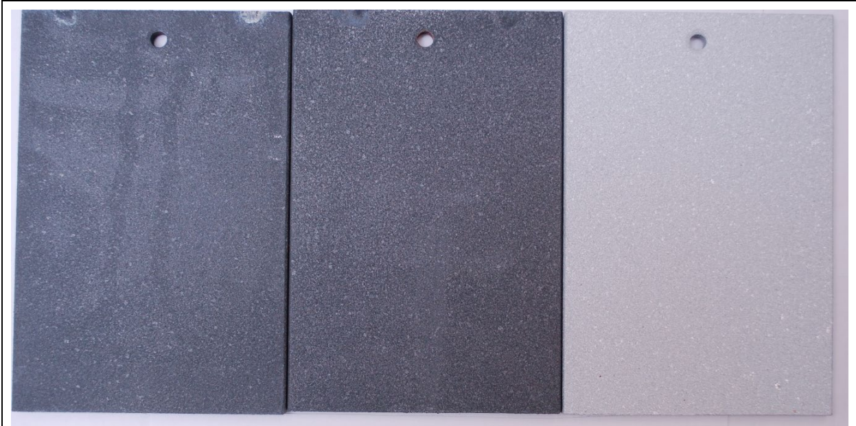
ZnAl TSC: Humidity exposed (L), Humidity exposed with pressure wash/blow dry (C), No exposure (R)
