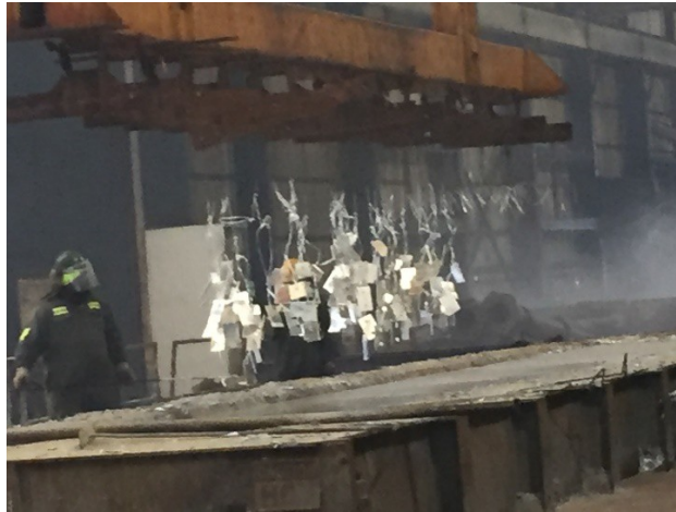
Figure 1-1. Test panels being removed from the galvanizing bath.
