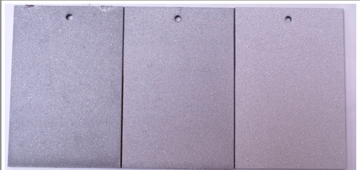
AI TSC: Humidity exposed (L), Humidity exposed with pressure wash/blow dry (C), No exposure (R)
