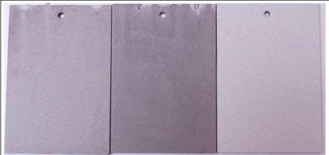
AI TSC: Humidity exposed (L), Humidity exposed with pressure wash/blow dry (C), No exposure (R)
