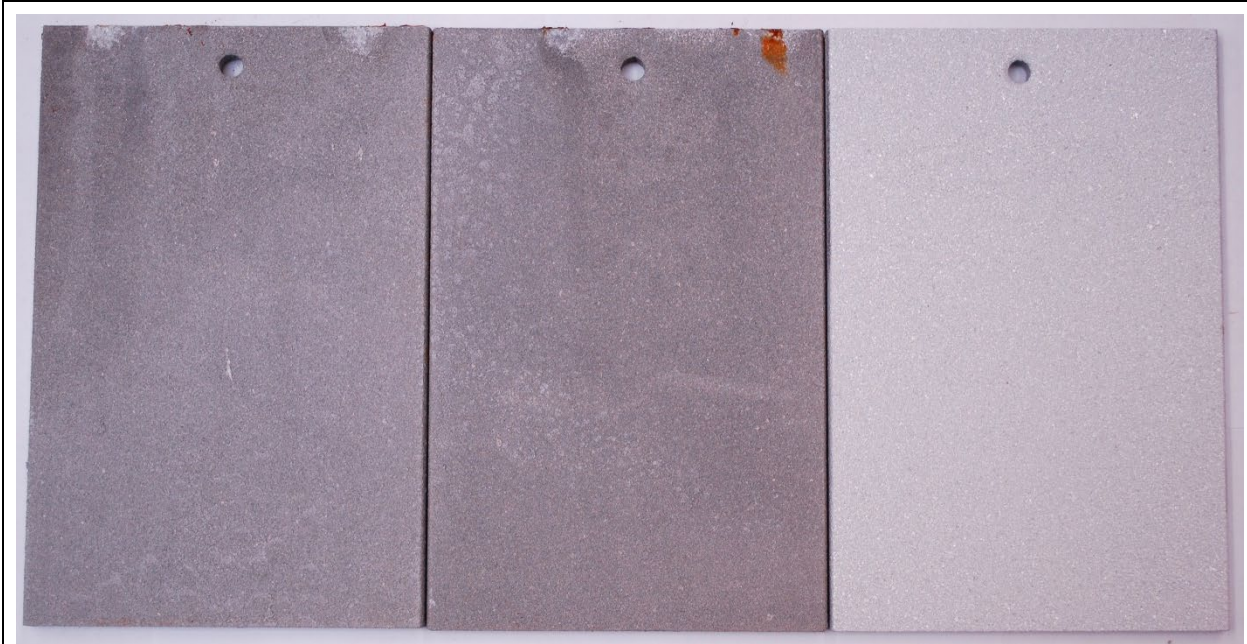
AI TSC: Humidity exposed (L), Humidity exposed with SP1 (C), No exposure
